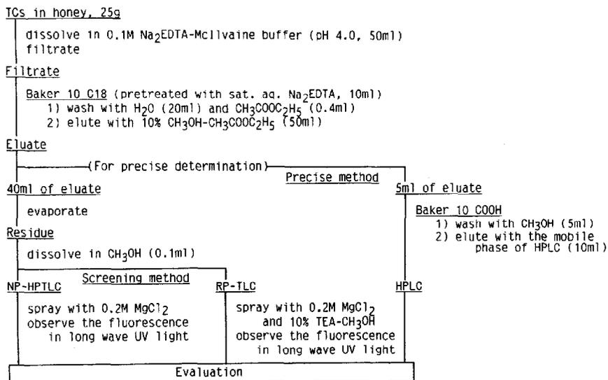
Scheme 1. Systematic analytical method for seven residual tetracyclines.
