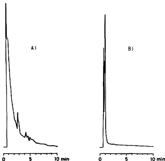
Fig. 4. Comparison of chromatograms before (A) and after (B) clean up on a Baker-10 COOH cartridge. For chromatographic conditions, see Experimental.
