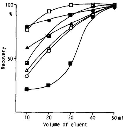
Fig. 3. Effect of the volume of 10% methanol in ethyl acetate solution on the recovery of seven tetracyclines from a Baker-10  $C_{18}$  cartridge. Procedure as in Fig. 2. For symbols, see Fig. 1.
