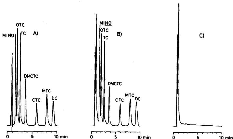
Fig. 5. Typical chromatograms of honey extracts. (A) standard of TCs (10 ng); (B) fortified honey (1.0 ppm); (C) blank of honey. For chromatographic conditions, see Experimental.
