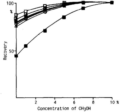
Fig. 1. Elution curves for seven tetracyclines from a Baker-10 COOH cartridge. After application of TCs ( $25 \mu\text{g}$  of each) in 1 ml methanol, they were eluted with various volumes of the mobile phase, methanol-acetonitrile- $0.01 M$  aqueous oxalic acid (2:6:16), pH 3.0, and then the recoveries were calculated. TCs; O, MINO; ●, OTC; △, TC; ▲, DMCTC; □, CTC; ■, MTC; □, DC.
